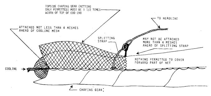
ANY MATERIAL MAY BE USED TO PROTECT THE BOTTOM OF CODEND
