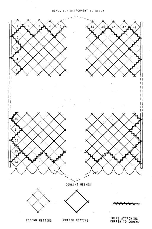
EXAMPLE 3 - CHAFER OF SINGLE-BRAIDED, THICK, KNOTLESS TWINE MATERIAL: MANNER IN WHICH THE CHAFER IS FITTED TO THE CODEND.
