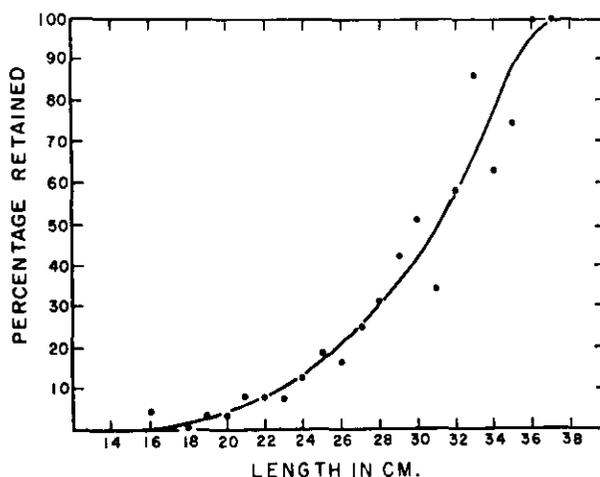
Fig. 1. Percentage of redfish of each length retained by a manila codend of 132 mm mesh size. (From data of Clark 1957e).
