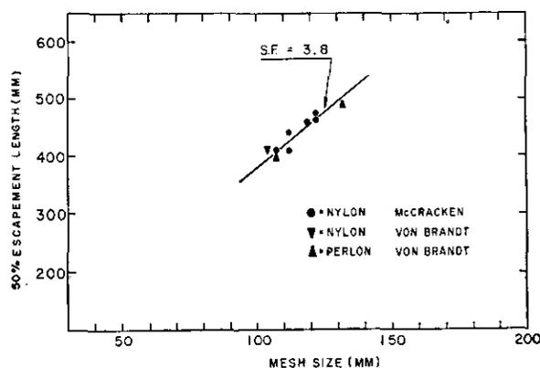
Fig. 10. Cod 50% retention lengths for nylon codends of both double and single strand construction and perlon codends of double strand construction.
