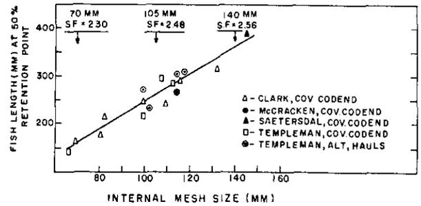
Fig. 6. Redfish 50% retention lengths for double manila codends, 45/4 - 125/3.
