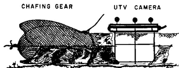
Fig. 1. Television camera rigged to study the effect of chafing gear on escapement from the codend.
