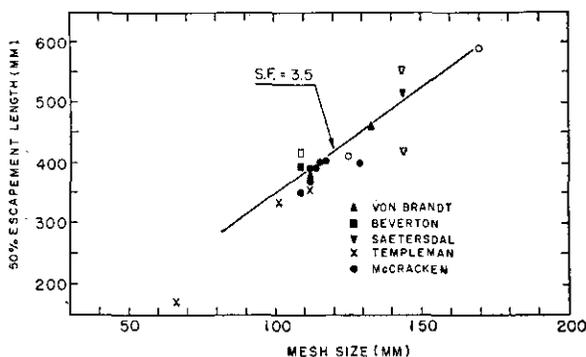
Fig. 9. Cod 50% retention lengths for manila codends of double strand construction. Open symbols represent results from experiments with less than 50 fish per tow in the selection range.
