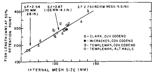
Fig. 7. Redfish 75% retention lengths for double manila codends, 45/4 - 125/3.
