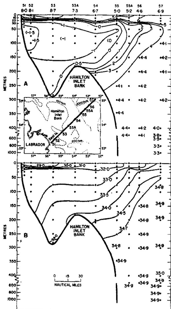
Fig. 2. Hydrographic section from Seal Islands, Labrador, across Hamilton Inlet Bank, Aug. 2-5, 1960. A—Temperature °C; B—Salinity per mille.
